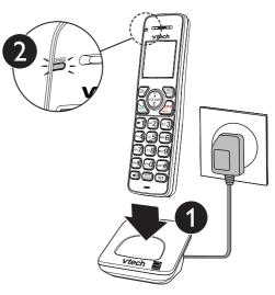
Once you have installed the battery, the handset LCD display indicates the battery status (see the table on next page).
